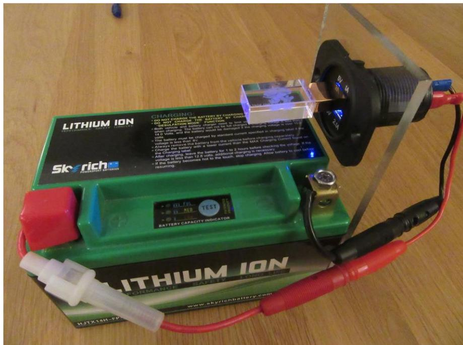
It is a 12V Lithium Ion battery and a 5V USB adapter. It appears to be an ideal power supply for the 5G key.
